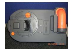
C Using the sliding cover as a lever rotate the complete mechanism anti clockwise until the arrow points to the second dot.
