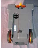
Place flat head screwdriver underneath rib and take one complete rib out, if not broken yet.
