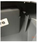
The float simply unclips and clips back into place, when replacing the float ensure the fin is positioned towards the base of the waste tank.
