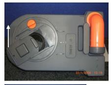
Return the sliding to cover to it's original position, fill the waste tank with clean water and test.
