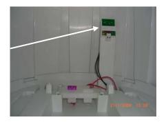
B Simply remove the reed switch by pulling it up and away from its housing at the top of the stem
