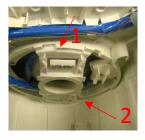
C Unscrew the three retainer brackets
