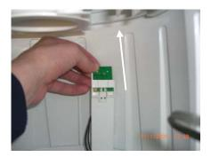
Replace the reed switch and ensure that it is correctly inserted into the wiring harness connection
