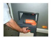
Remove the waste holding tank and pull out the drain tube from its retaining bracket.
