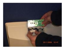
Clip the control panel back into its housing and clip the two parts back in the toilet
