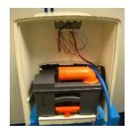
B Remove the bowl retainer brackets.(2x) Turn #1 anti-clockwise and #2 clockwise to remove
