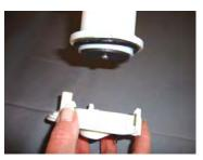
Place new pump retainer and press it back onto the pump.
