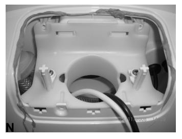
Replace the bezel. If required use some of the PTI sealant provided ensuring a nice clean seal.
