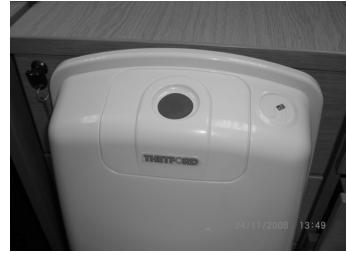
Use a paint scraper type object (use a cloth around the scraper if necassary to prevent damage to the toilet) and lever up the bezel, slowly working the bezel free all the way round. Illustration C
